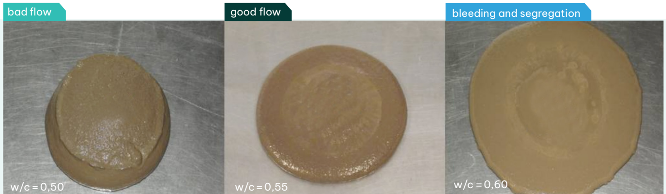
Figure 4: from left to right: bad flow, good flow, bleeding and segregation
