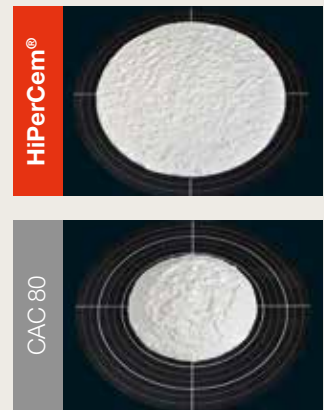
Flow Behaviour Standard Castable
